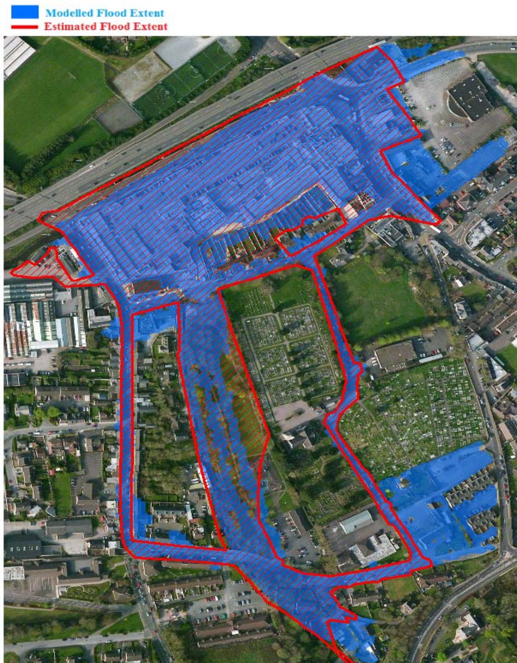
Figure 8.2: June 2012 flood extent calibration plot (maximum flood extent vs maximum modelled flood event). Area 2 (Tramore River through St Patrick’s Mills, Douglas) and Area 1 (Ballybrack Stream through Douglas) are located to the north west and the south of this figure, respectively. The N40 (South Ring Road) runs along the northern boundary of the figure. Source: Cork County Council.
